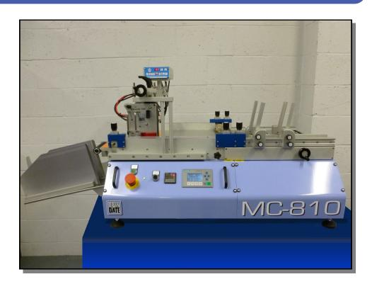
The MC810 is an automatic feeding system suitable for a wide range of flat items including paper labels, cards, sleeves, cartons, crash lock cartons and skillets. When fitted with a hot foil, thermal transfer or inkjet printer or a deboss coder from our comprehensive range it provides an extremely versatile, off-line, stack to stack overprinting facility.
