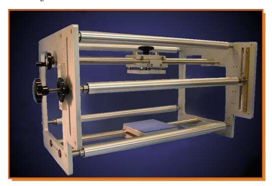
The system comprises of rollers, print registration units and tie bars of varying lengths, end plates, base plates and printer mounting plates etc. which can be assembled, dismantled and reassembled as necessary so that the requirements of the packaging machine, pack, customer and printer are best met
