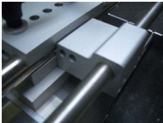
Secure the block to the printer with 2 off M5 screws
