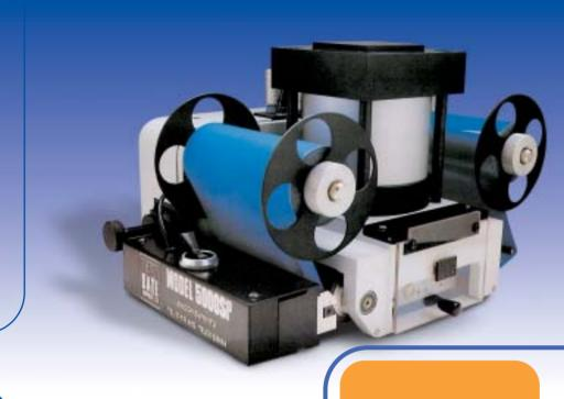
The Open Date 5000 Series automatic hot foil overprinters are high quality heavy duty machines. They are designed to be attached to reel fed packaging machines providing a large area on-line printing facility for logos, graphics, dates, prices, batch codes, ingredients lists, bar codes etc.
