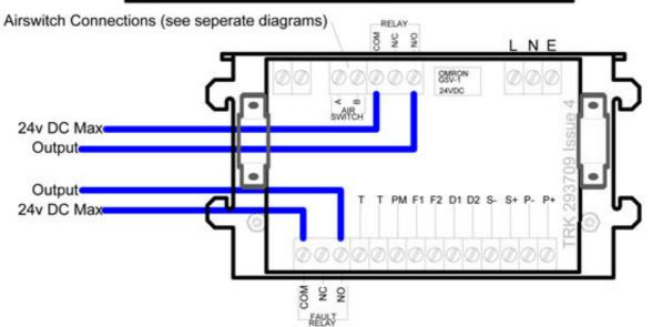
Print Relay:- Rated 24v DC, 1 amp max current
