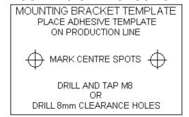
Locate the supplied mounting template and affix in a convenient location on the production line. Spot and drill both mounting holes for an M8 screw. NOTE: the user may also thread the side of the conveyer using an M8 tap.
