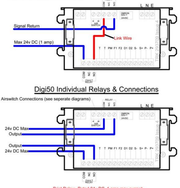
Print Relay:- Rated 24v DC, 1 amp max current
