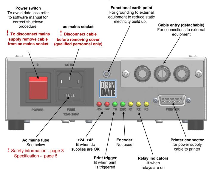
Power switch; Before switching off the software must be put into standby to avoid data loss.
