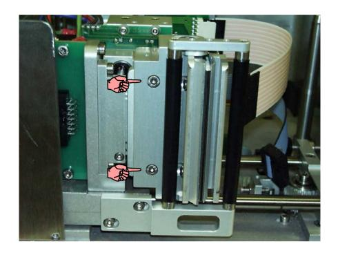
Undo and remove cap screws.
