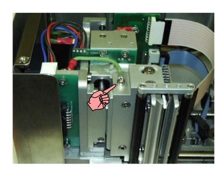
Undo and remove earth lead retaining cap head.
