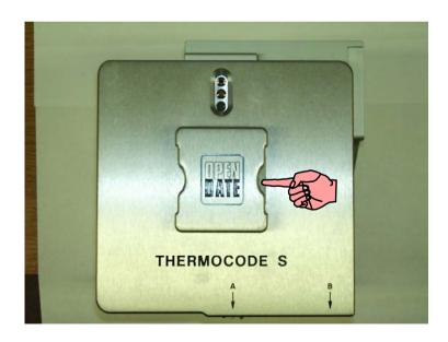
Push in latch and remove ribbon cassette from print head assembly.
