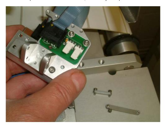
Take care not to damage the ribbon cable in the retaining clamps
