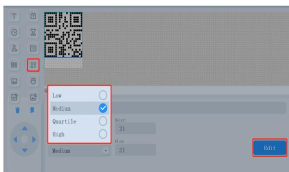
Click **User Field-2D Code**, and add the module of QR Code. It supports QR CODE and DMatrix. The height and width of the QR code are system default and vary with different categories. This machine supports up to 78 characters.
