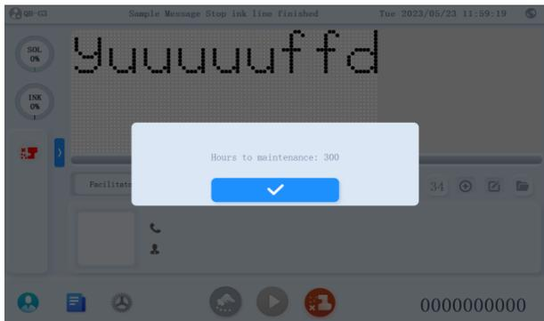
When remaining time is equal to 0 hour, start the printer and then the prompt message of "0 hour" will appear. The printer cannot start printing. If it happens when printing, close the dialog box and then the printer continues to print. If you stop printing at this point, it will not restart.
