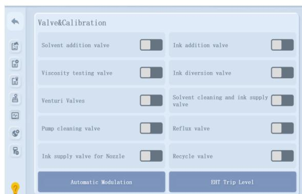
**Valve Test:** Click switch button of any valves, it will proceed switch on/off operation, to monitor if the valves are work normally.
